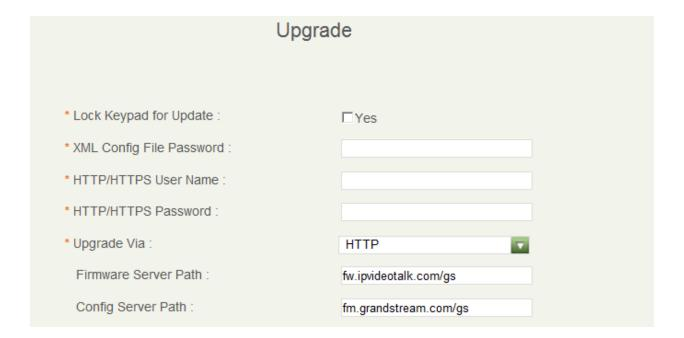
Figure 2: Using web UI to define the XML Configuration File Password
