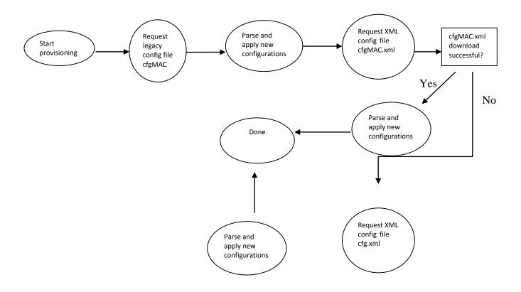
Figure 1: Provisioning Flow.
