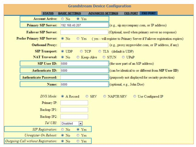
Figure 15: Method 2 - Configure FXO Port on the HT503: Registration
