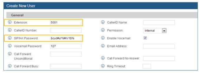
Figure 2: Method 1 - Create Extension 5001 on the UCM6100
