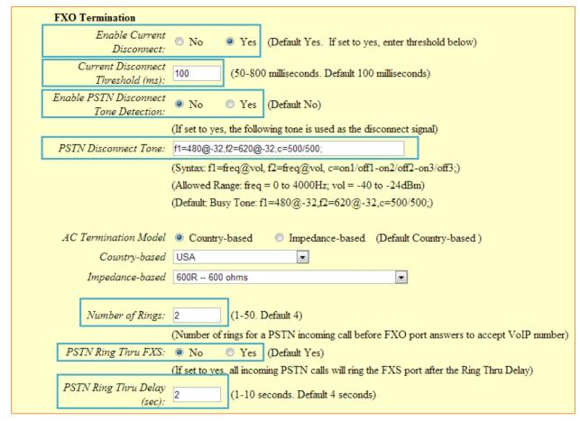
Figure 17: Method 2 - Configure FXO Port on the HT503: FXO Termination
