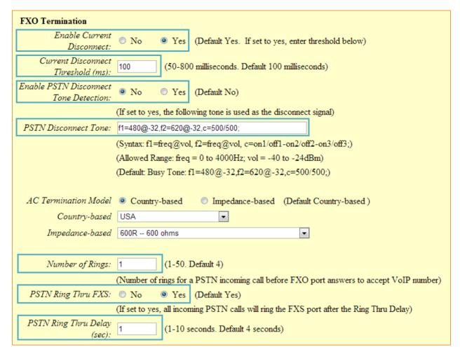
Figure 7: Method 1 - Configure FXO Port on the HT503: FXO Termination
