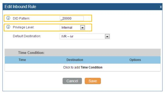
Figure 14: Method 2 - Configure Inbound Rule on the UCM6100
