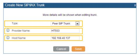
Figure 12: Method 2 - Create Peer SIP Trunk on the UCM6100
