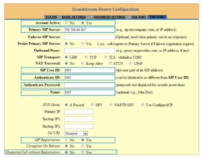
Figure 5: Method 1 - Configure FXO Port on the HT503: Registration
