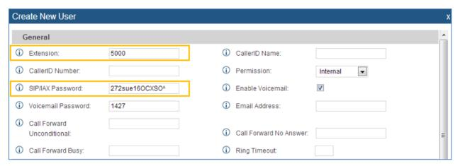
Figure 1: Method 1 - Create Extension 5000 on the UCM6100
