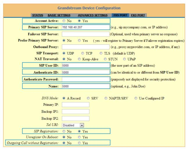
Figure 4: Method 1 - Configure FXS Port on the HT503
