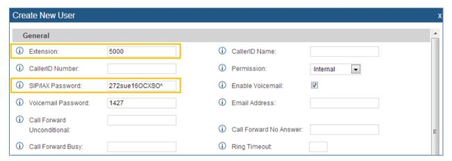
Figure 10: Method 2 - Create Extension 5000 on the UCM6100
