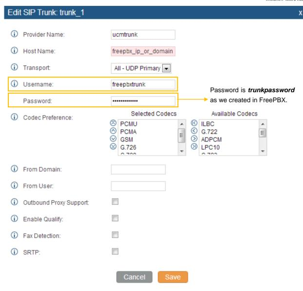
Figure 5: Configure Register SIP Trunk on the UCM6100
