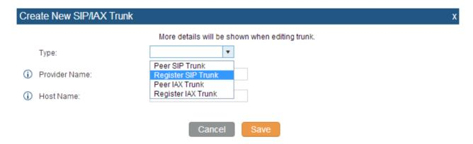
Figure 4: Create Register SIP Trunk on the UCM6100
