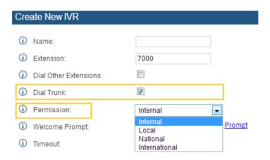
Figure 5: Create an IVR on UCM6100 - Dial Trunk Enabled
